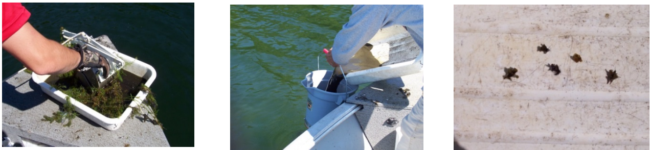
Figure 32. Ponar sediment sample (left), sieve separation of sediment (middle), and turions collected (right).
